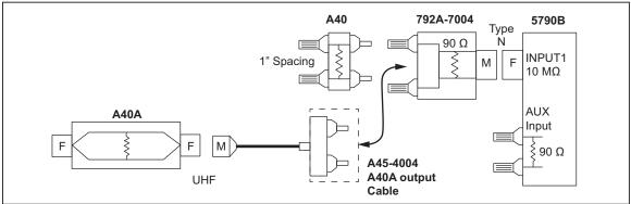
Figure 4-4. Measuring Relative Current Using 792A-7004
