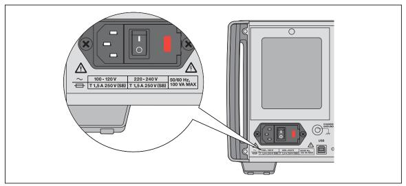
Figure 2-2. Line Power Label and Switch Location
