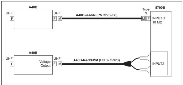
Figure 4-3. Measuring Absolute Current Using A40B
