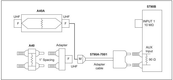
Figure 4-5. Measuring Relative Current Using 5790A-7001
