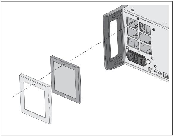
Figure 7-2. Accessing the Air Filter
