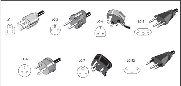
Figure 2-1. Line Power Cord Types Available from Fluke
