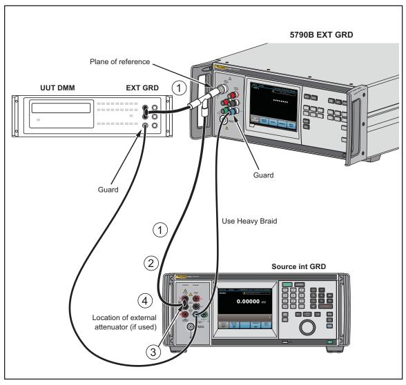
Figure 4-1. Recommended Test Lead Connections to Test a Voltmeter
