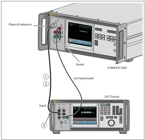
Figure 4-2. Recommended Test Lead Connections to Test a Source
