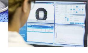
The uniform LED lighting and high-quality optical components ensure that the dispensed drop is portrayed with the correct shape. Reliable and accurate contact angle measurements can be achieved with the aid of the particularly fast and high-resolution USB 3.0 camera.
