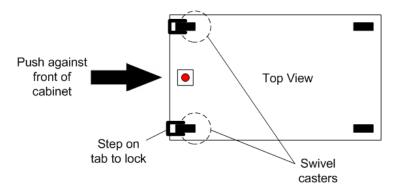
Once the cabinet is placed in its final location, lock the front casters by stepping on the locking tab. This will prevent the cabinet from moving.
