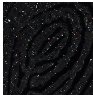
Leica LED5000 MCI™: The same sample in flat incident light. Clearly visible: dust particles
