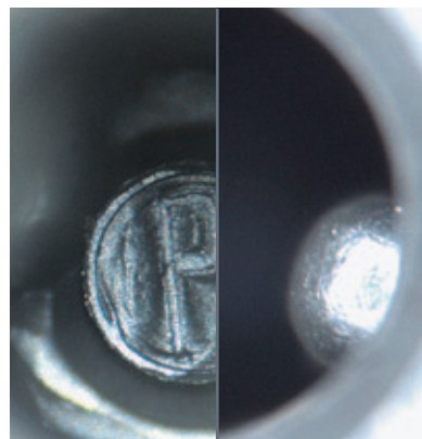
Enlarged detail of an injection nozzle – left: with Leica LED3000 NVI™, right: with conventional ring light
