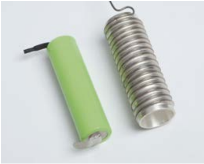
18650 cell and its VariPhi® 3-D sensor
