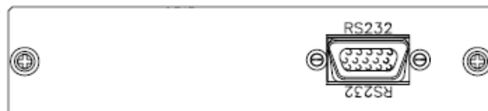
Fig 2-4 1000A RS232 Connection
