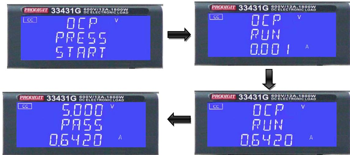
5.11.1.8. the UUT's output voltage drop-out lower than the threshold voltage(V-th setting), and the OCP trip point is between I\_Hi and I\_Lo limitation, then middle 5 digits LCD display will shows "PASS", otherwise shows "ERROR".
