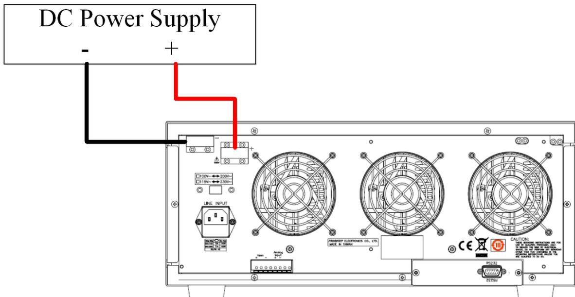
Fig 5-1 Local voltage sense connections
