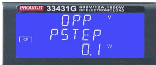
5.12.1.5. Press up key, set stop load watt 3.2W, press OPP key to the next step.
