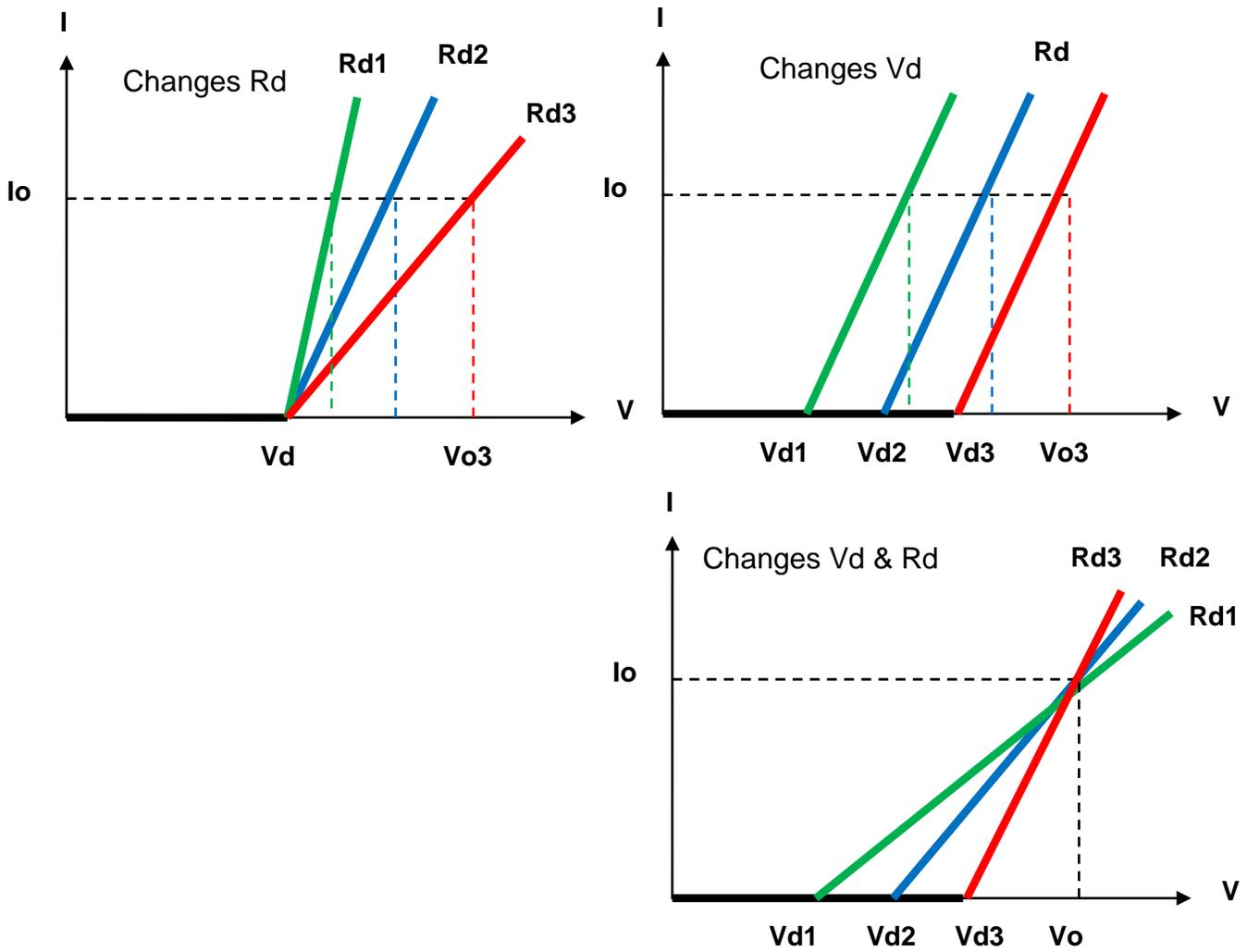
Fig 5-12 LED MODE operation mode of the application
