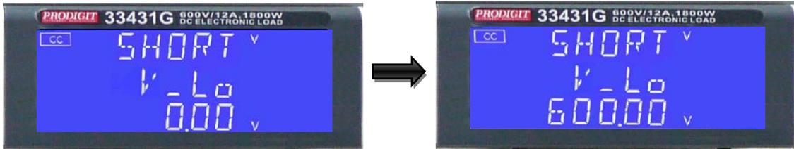
Note. The V-Hi and V-Lo parameter is difference with the V-Hi and V-Lo in the LIMIT function.
