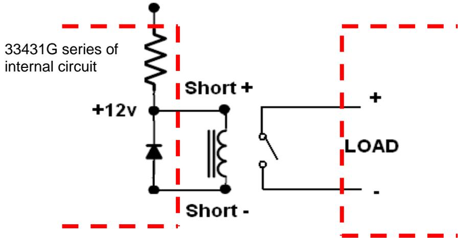
Fig 5-17 short test connection
