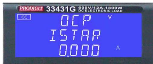
5.11.1.4. Setting step load current 0.001A, press OCP key to the next step.
