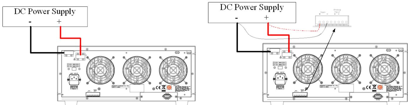
Fig 3-2 typical connection of 33431G series load
