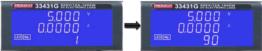
Note: Changing the quantity of possible shift caused Rd, Rd automatically switch to The original settings, if you have exceeded the value of the nearest range setting, Change the quantity of confirmed again after the settings are correct.
