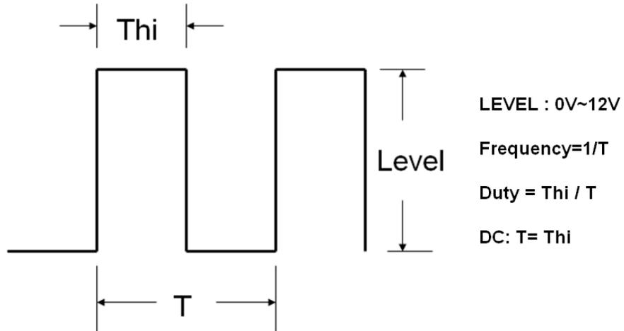
Fig 3-3 33431G Series Electronic Load DIMMING CONTROL(PWM TYPE)
