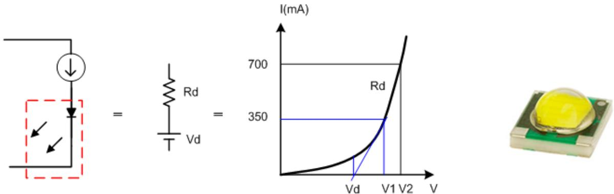
Fig 5-8 LED's equivalent circuit and characteristic curve
