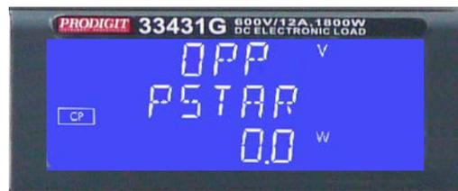
5.12.1.4. Press up key, set step load watt 0.1W, press OPP key to the next step.
