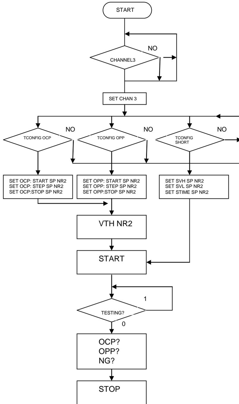
Fig 5-16 33431G series electronic load OCP, OPP, SHORT operation flow chart
