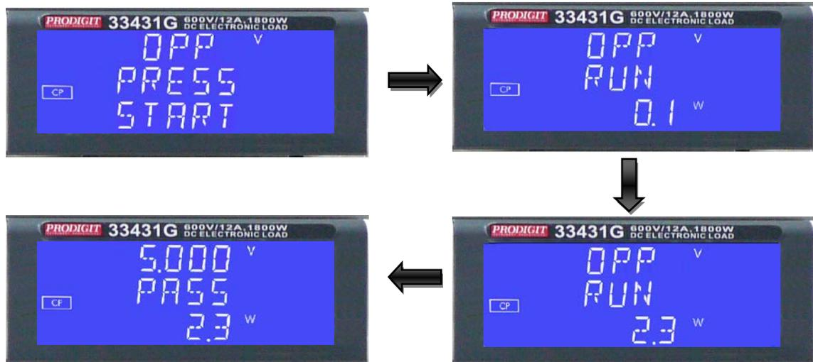
5.12.1.8. The UUT's output voltage drop-out lower than the threshold voltage ( $V_{th}$  setting), and the OPP trip point is between  $W_{Hi}$  and  $W_{Lo}$  limitation, then lower 5 digits LCD display will shows "PASS", otherwise shows "FAIL".
