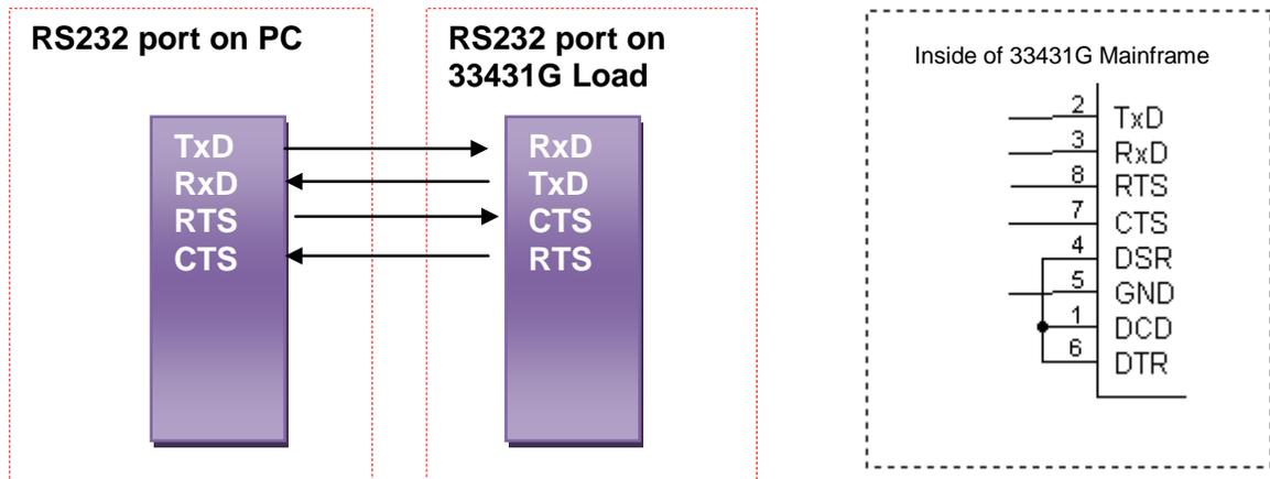
Fig 4-1 RS-232C INTERFACE CONNECTION OF REAR PANEL
