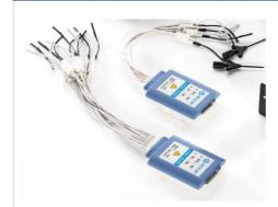
The digital inputs are grouped into logic probes with eight channels. High input impedance combined with low input capacitance of 100 k $\!\Omega$  II 4 pf ensures high signal fidelity and low loading of the test points.
