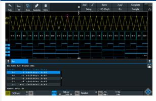
The R&S®RTx-B1 option supports 16 digital channels and simultaneous decoding of up to four parallel buses. Each bus is represented by a line on the edge of the screen.
