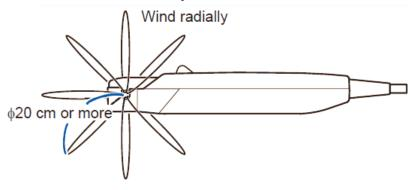
Cord placement and the act of clamping the probe onto the conductor being measured may trigger load fl uctuations, affecting the observed waveform.
