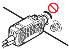
Demagnetizing and Zero Adjustment
