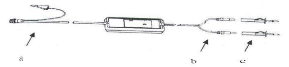
a. Output cable The BNC output connector and an auxiliary grounding
