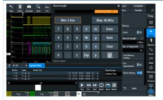
The history and segmented memory offer various user options, providing more flexibility for your applications. Automatic and manual memory configuration are available. In automatic mode, the instrument automatically defines the record length (number of waveform samples that are stored) and the number of history segments. In manual mode, you can set these parameters yourself.
