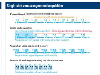
Long data sequences are usually acquired in a seamless single shot. With a maximum record length of only a few milliseconds, acquisition is often limited to a single event or protocol packet. The memory can be divided into several steps. When the fast segmented memory mode is activated, the blind time is reduced to  $0.5~\mu s$ .
