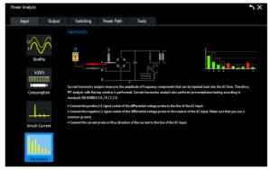
After you select a measurement function, the measurement wizard guides you through the test setup. Detailed illustrations help you make the correct connections. The oscilloscope then configures itself automatically and delivers quick results. You can modify the configuration or completely manually configure the oscilloscope in order to document specific signal details.
