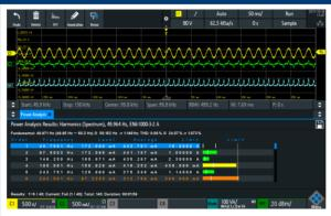
Different standards for limiting the harmonic current must be met when developing switched-mode power supplies. The R&S\*RTx-K31 power analysis option helps you test all common standards: EN 61000-3-2 classes A, B, C, D, MIL-STD-1399 and RTCA DO-160.
