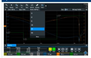
Choose the points per decade to set up and modify the resolution of your plot. The oscilloscope supports up to 500 points per decade. Drag markers to the desired position directly on the plotted trace and easily determine the phase and gain margin.
