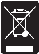
Fig. 1.2: Product labeling in accordance with EN 50419
