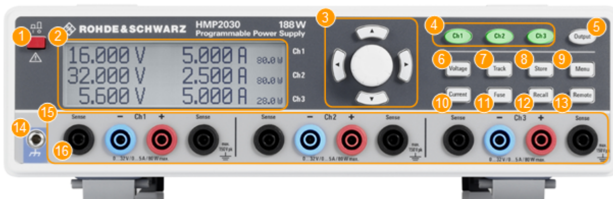
Figure 3-1: Front view of the R&S HMP2030
