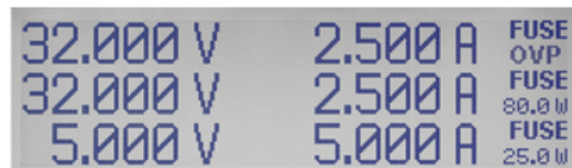
Figure 4-6: Overvoltage protection (example R&S HMP2030)
