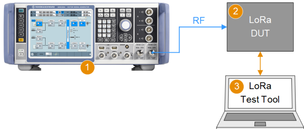
Figure 6-1: Test setup for Rx sensitivity test
