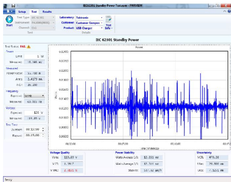
IEC62301 Standby power testing with real-time uncertainty and stability measurements
