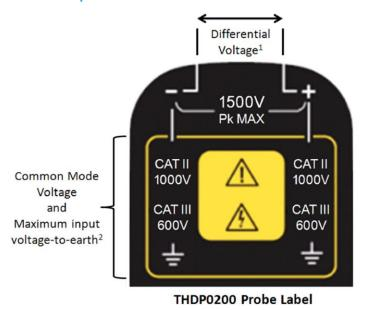
1. The differential voltages the maximum measurable range between the (+) and (-) input leads of the probe. Beyond these limits, the output could be clipped.
