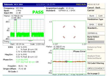
Option VM02 GSM-EDGE, ( $3\pi/8$  8PSK, 270.833 kS/s, 935 MHz, 0 dBm), RMS EVM: 0.30%
